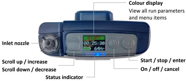
Blue light flashes when pump running Red light flashes when there is a fault or during charging
